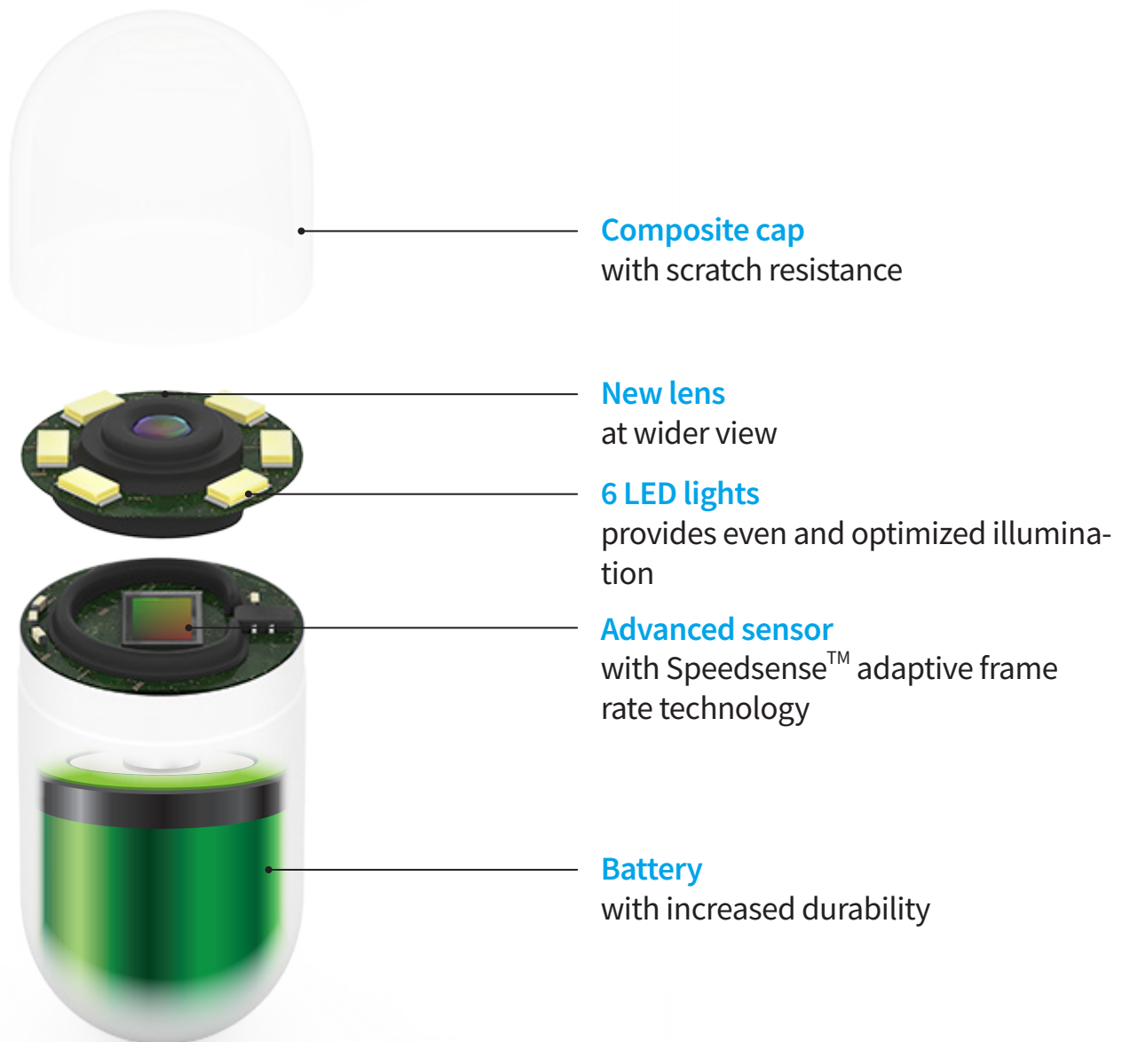
OMOM Capsule Structural Illustration
